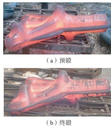
图3 飞机起落架外筒2火次模锻成形方案 [23] Fig.3 Two-stage die forging forming scheme of outer barrel of aircraft landing gear [23]
